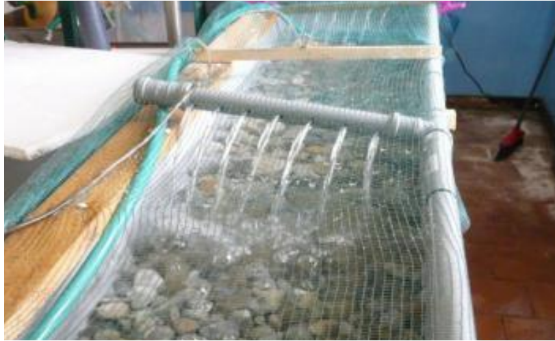
Figure 5. Turbulence is created by leaky pipes.
